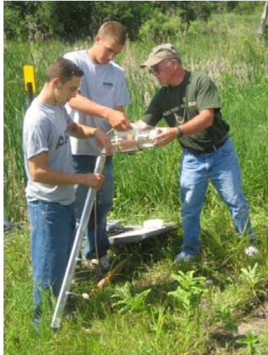
Win E Mac High School River Watch Students utilizing a 100 cm transparency tube to measure clarity in the Red Lake River Watershed.
